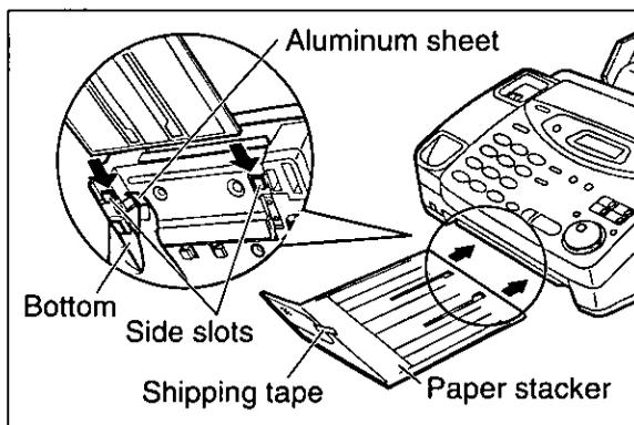
**3** Confirm that the paper stacker is locked into the center slots and slide back.
