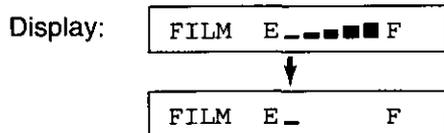
When the film indicator points to this position, the remaining film will print up to 25 pages of letter size document. Prepare a new film cartridge for replacement.
